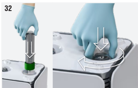
Fig. 32: Screw the new ionizing tubes back into place by acting again on the glass surface that can be reached by hand through the special slots.
