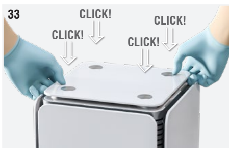
Fig. 33: Put the lid back on the device by pushing it until the parts are locked in place.
