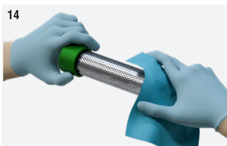
Fig. 14: Clean the glass using a damp cloth.
