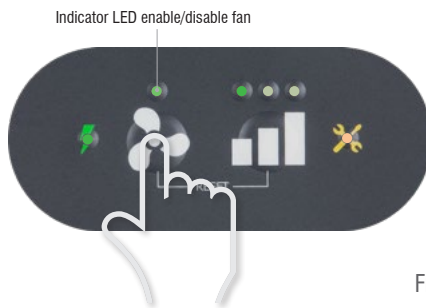
Fig. 9: Press the 🌀 button to activate or deactivate the ventilation function.
