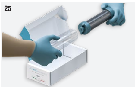
Fig. 25: Unpack the new ionization tube by handling it carefully as it is fragile.
