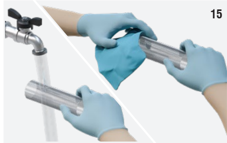
Fig. 15: Wash the mesh under running hot water and dry it thoroughly with a non-fraying cloth.
