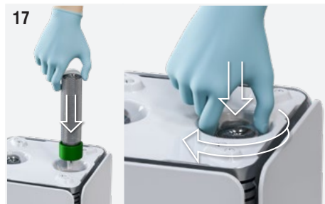
Fig. 17: Screw the ionizing tubes back into place by acting again on the glass surface that can be reached by hand through the special slots.
