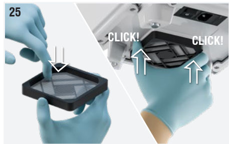
Fig. 25: Put the mesh filter back into the filter cover. Reassemble the filter cover with the snap fastening. Press it on the grid incorporated in the closing plate until you feel the snap of the coupling between the parts.
