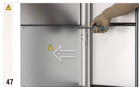
Fig. 47: Reposition the panel that protects the fan using the retaining screws.
