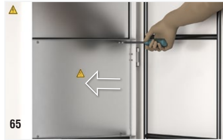
Fig. 65: Reposition the panel that protects the fan using the retaining screws.
