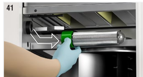
Fig. 41: Gently unscrew the ionising pipe, gripping it at the base (green part). If the operation is difficult to perform, pull slightly the earthing spring so that it is not in contact with the surface of the tube.
