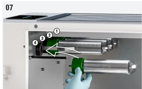
Fig. 7: Gently screw the tubes ionizing by grasping them at the base (part green). If the operation is difficult to perform, pull slightly the earthing spring so that it is not in contact with the surface of the tube.
