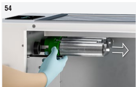
Fig. 54: Gently unscrew the ionising pipe, gripping it at the base (green part). If the operation is difficult to perform, pull slightly the earthing spring so that it is not in contact with the surface of the tube.
