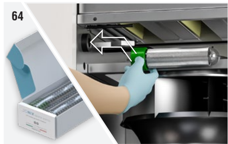
Fig. 64: Gently screw in the new ionising pipe , holding on to the base (green part). If the operation is difficult to perform, pull slightly the earthing spring so that it is not in contact with the surface of the tube.
