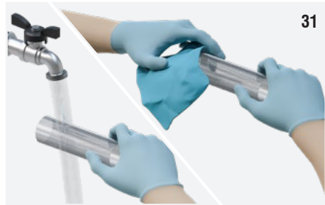
Fig. 31: Wash the mesh under running hot water and dry it thoroughly with a non-fraying cloth.
