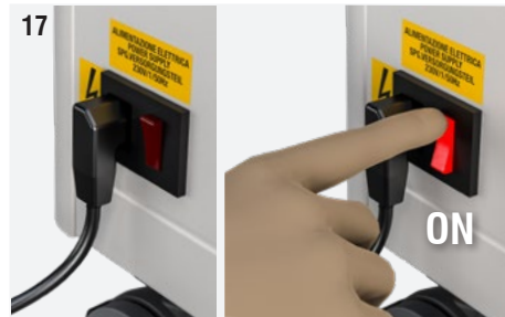
Fig. 17: In order to turn on the device move the red switch up. The switch lights up, indicating that the device is on.
