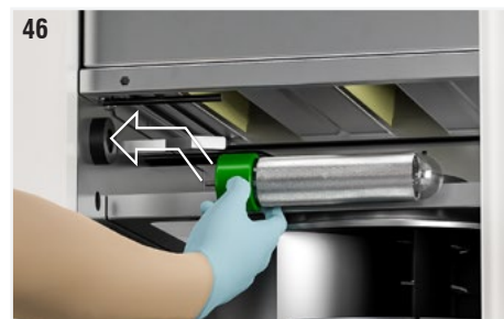
Fig. 46: Gently screw the ionising tube holding on to the base (green part). If the operation is difficult to perform, pull slightly the earthing spring so that it is not in contact with the surface of the tube.
