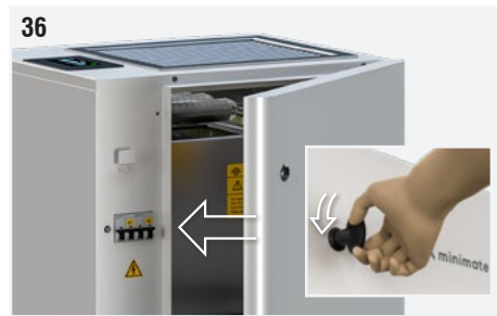
Fig. 36: Close the front maintenance access panel with the maintenance access key.
