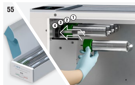
Fig. 55: Gently screw in the new ionising pipe , holding on to the base (green part). If the operation is difficult to perform, pull slightly the earthing spring so that it is not in contact with the surface of the tube.
