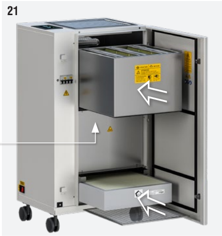
Fig. 21: Put the new / clean filters back in place. Push the filter locking tabs inwards until they click.
