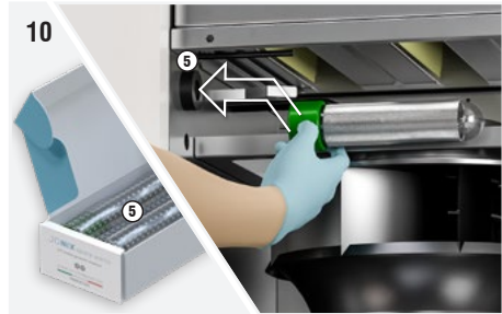
Fig. 10: Gently tighten the ionising pipe by gripping it at the base (green part), positioning it in its seat above the fan. If the operation is difficult to perform, pull slightly the earthing spring so that it is not in contact with the surface of the tube.
