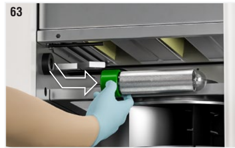
Fig. 63: Gently unscrew the ionising pipe, gripping it at the base (green part). If the operation is difficult to perform, pull slightly the earthing spring so that it is not in contact with the surface of the tube.
