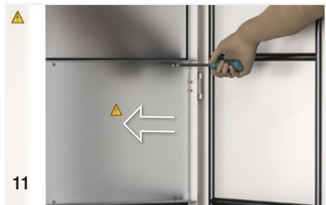
Fig. 11: Reposition the panel that protects the fan using the retaining screws.
