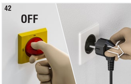
Fig. 42: Switch the device off by turning the switch. Remove the plug connected to the mains.
