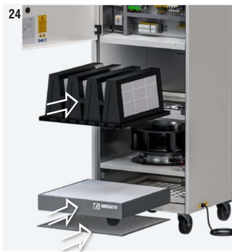
Fig. 24: Put the new / clean filters back in place. Push the filter locking tabs inwards until they click..
