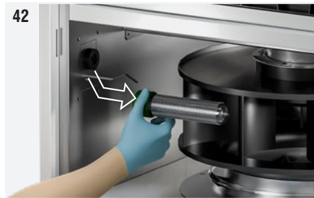
Fig. 42: Gently unscrew the ionising pipe, gripping it at the base (green part). If the operation is difficult to perform, pull slightly the earthing spring so that it is not in contact with the surface of the tube.
