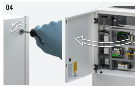
Fig. 4: Use a screwdriver to open the top rear panel.
