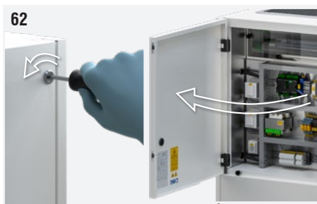
Fig. 62: Use a screwdriver to open the top rear panel.
