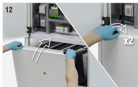
Fig. 12: Put the cover panel back in place. Screw the knobs back on.
