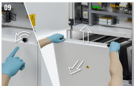
Fig. 9: Unscrew the 2 knobs which keep the rear bottom panel for maintenance access. Lift and then pull you towards to remove the panel.
