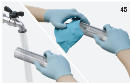
Fig. 45: Wash the mesh under running hot water and dry it thoroughly with a non-fraying cloth.
