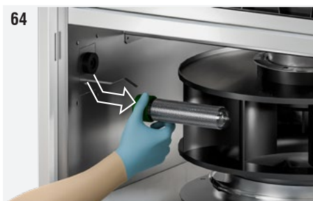
Fig. 64: Gently unscrew the ionising pipe, gripping it at the base (green part). If the operation is difficult to perform, pull slightly the earthing spring so that it is not in contact with the surface of the tube.
