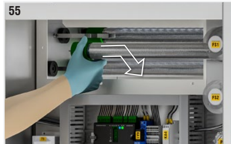
Fig. 55: Gently unscrew the ionising pipe, gripping it at the base (green part). If the operation is difficult to perform, pull slightly the earthing spring so that it is not in contact with the surface of the tube.
