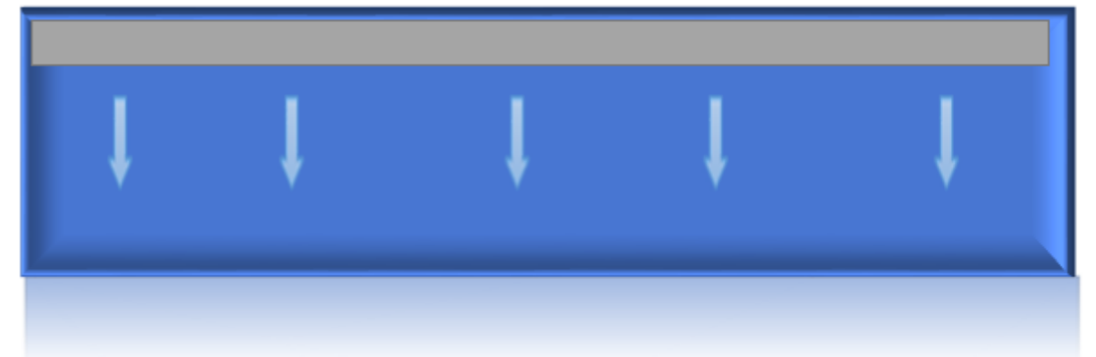
Figure 2 Front view of the room. Upper grid, dimensions: 0.5 x 13 m = 6.5 m 2 . surface of the opening. Open continuously, the result is a volume of incoming air equal to 2.764 m 3 /h.
