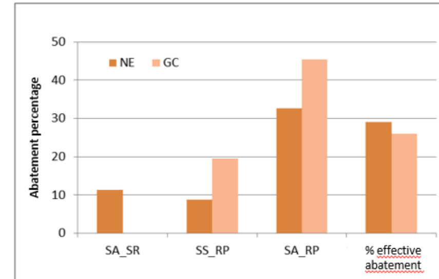
Figure 28. Results of tests conducted on MIX waste expressed as abatement percentages, taken at the sampling points 1 and 3. Legenda: SA_SR = % probe contribution; SS_RP = % decrease due to waste emission losses along the way; SA_RP = % abatement incorrect probe; % effective abatement = SA_RP – SS_RP – SA_SR
