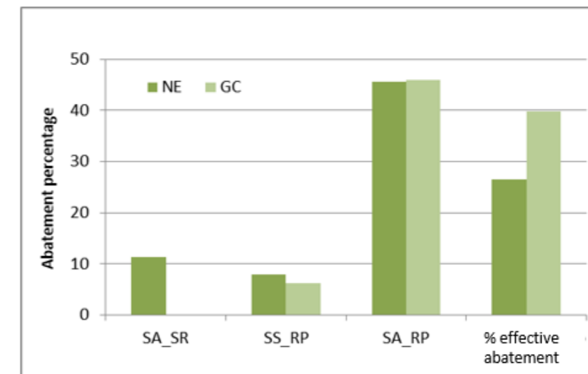
Figure 28. Results of tests conducted on LA waste expressed as abatement percentages, taken at the sampling points 1 and 3.
