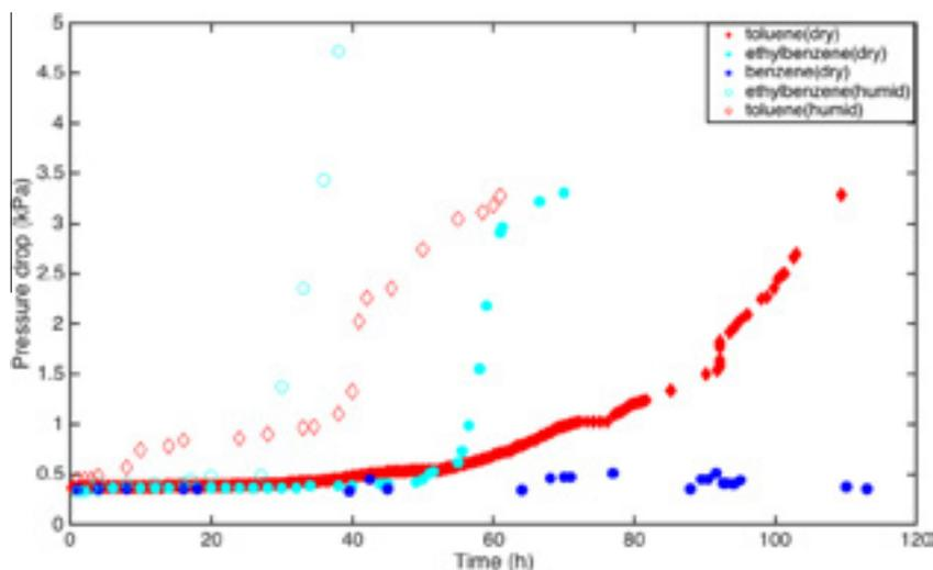
**Fig. 6.** Pressure drop determined as a function of time. Experimental conditions were 360 J L<sup>-1</sup> SIE, a gas flow rate of 6.6 L min<sup>-1</sup>, and 100 ppm<sub>v</sub> inlet concentration.
