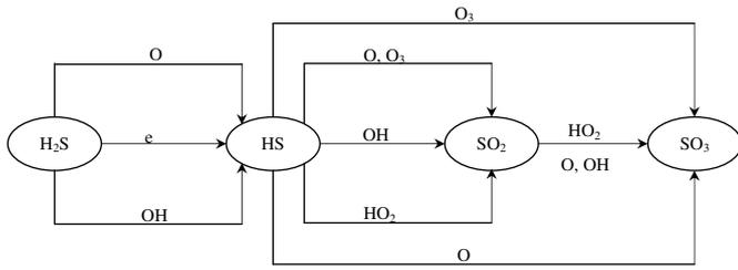
Fig. 13. Dominant pathways leading to the destruction of H<sub>2</sub>S molecules.
