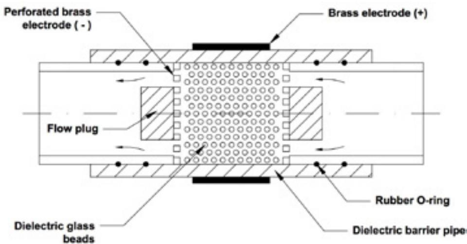
Figure 2. Schematic of the DBD packed-bed reactor.
