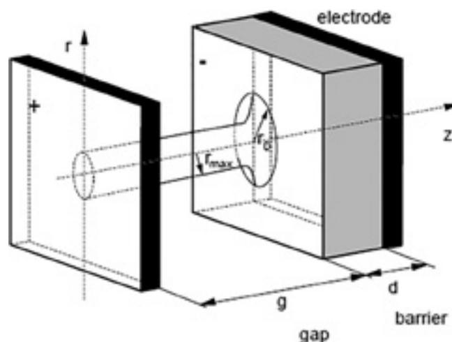
Fig. 5. The shape of a single microdischarge [64].
