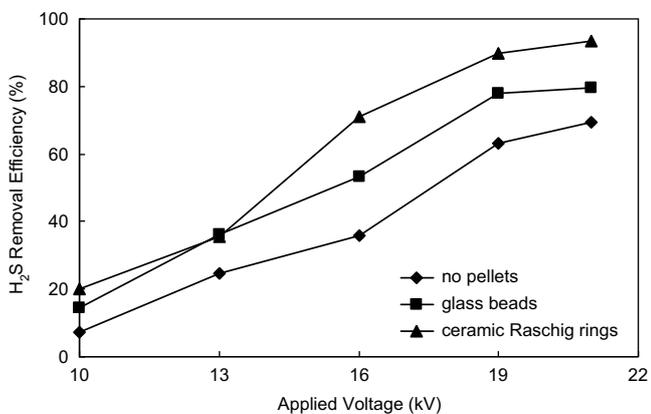
Fig. 10. H<sub>2</sub>S removal as a function of applied voltage for different reactors inlet concentration was 30 ppm; gas residence time was 0.8 s; and frequency was 300 Hz.
