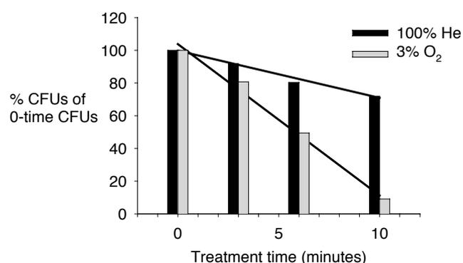
Fig. 10. Percent of surviving *Bacillus* spores vs. plasma treatment time for helium (black) and helium/oxygen mixture (97% He, 3% O<sub>2</sub>) (gray).
