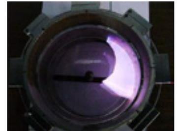
Figure 2. Magnetically Rotated Gliding Arc
