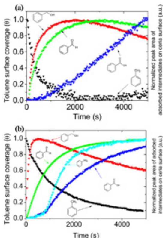
Fig. 13. Evolution of toluene and adsorbed intermediates surface coverage on CeO<sub>2</sub> as a function of post situ (a) and in situ (b) NTP exposure time [175].
