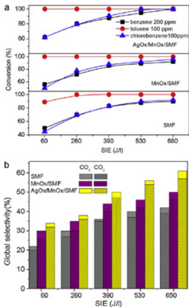
Fig. 5. Activity of SMF electrodes for higher VOC concentrations. (a) Conversion and (b) selectivity to CO<sub>x</sub> and CO<sub>2</sub>.
