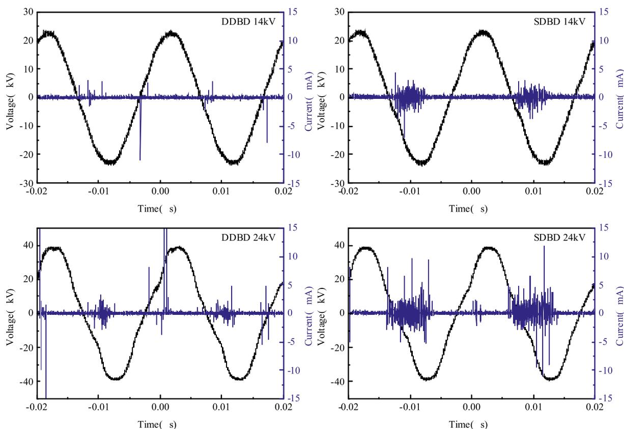
Fig. 7. Voltage and current waveform of DDBD and SDBD.
