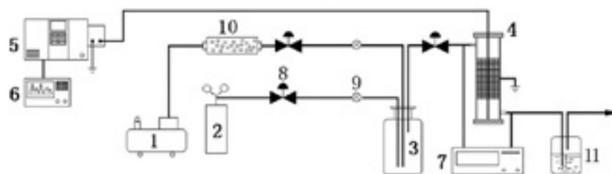
Fig. 1. Schematic diagram of the experimental setup 1. Air compressor 2. H<sub>2</sub>S gas cylinder 3. Mixing chamber 4. DBD reactor 5. AC power supply 6. Oscillograph 7. Spectrophotometer 8. MFC 9. Needle valve 10. Gas filtration system 11. Absorbent.
