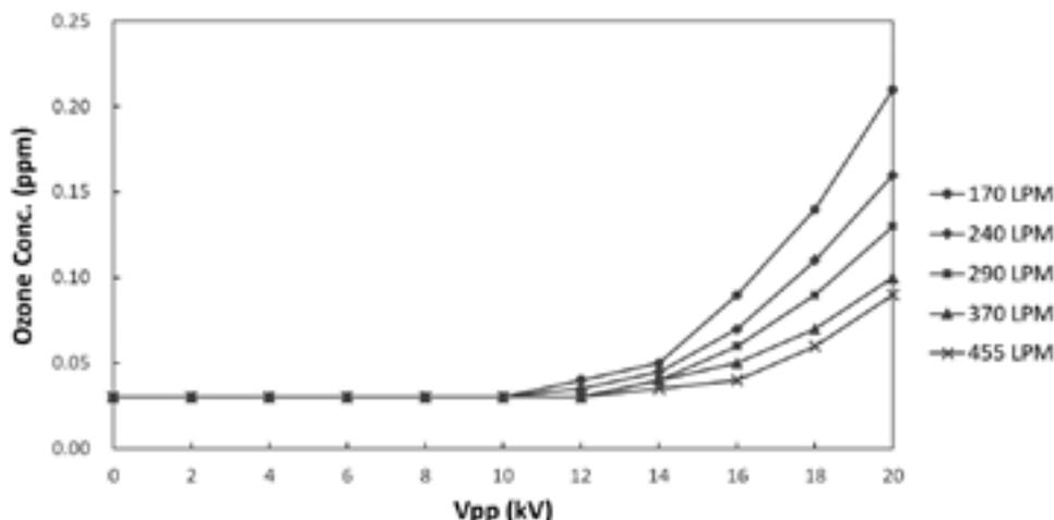
Figure 8. Measured ozone concentrations upstream of the ozone filter as a function of V<sub>pp</sub> and air flow rate.
