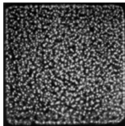
Fig. 4. End-on view of microdischarges in atmospheric-pressure air [51].
