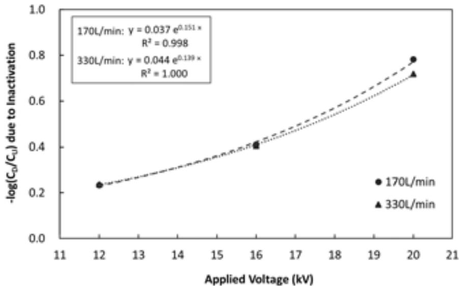
**Figure 7.** Log-reduction of infectious MS2 in airstream due to inactivation of the packed-bed NTP reactor activated by the variable voltage amplifier at 12kV, 16kV and 20kV ( $C_D$  and  $C_U$  represent the downstream and upstream concentrations in air, respectively).
