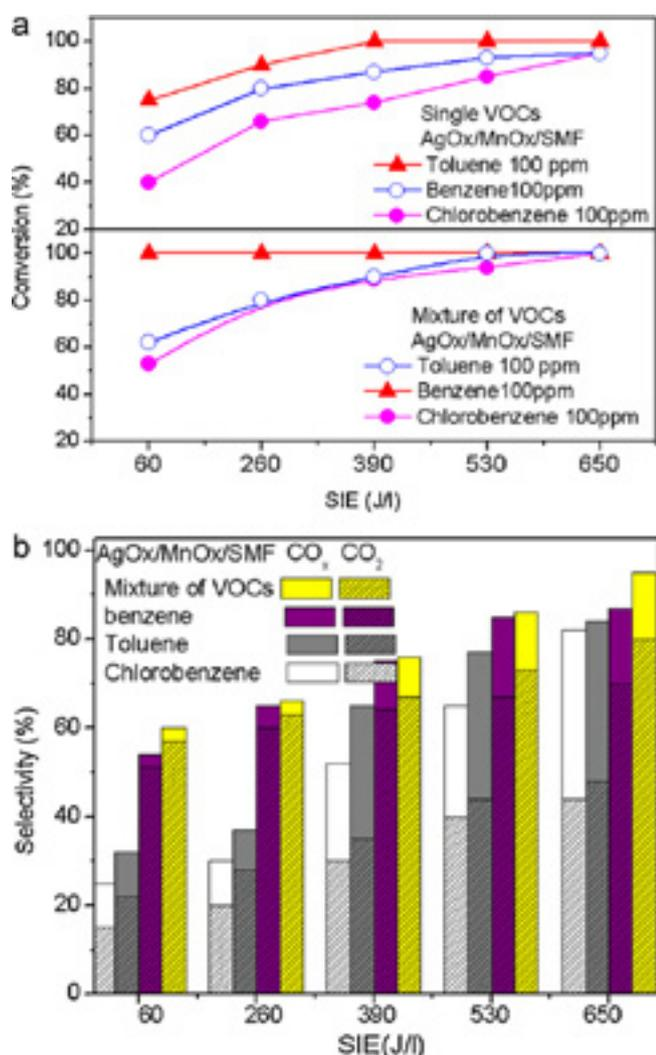
Fig. 4. Influence of single VOCs and mixture of VOCs on AgO<sub>x</sub>-MnO<sub>x</sub>/SMF electrode. (a) Conversion and (b) selectivity to CO<sub>x</sub> and CO<sub>2</sub>.
