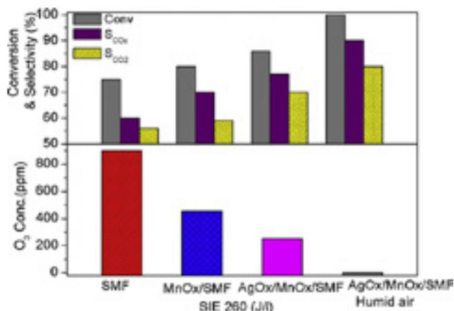
Fig. 3. Activity of SMF electrodes in plasma reactor during ozone decomposition with dry and humid air and influence of ozone concentration in the reactor on decomposition of mixture of VOCs at 260 J/l.
