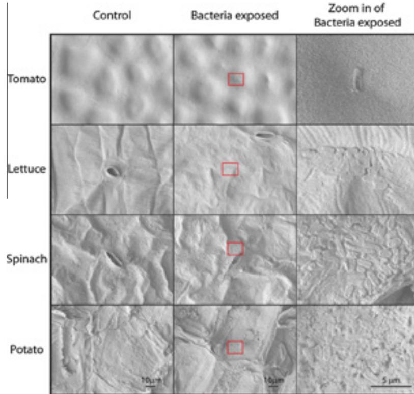
**Fig. 4.** SEM micrographs of four produce surfaces with or without exposing to bacteria dispersion for 5 min. Red rectangles indicates the areas from which higher magnification images were obtained. (For interpretation of the references to color in this figure legend, the reader is referred to the web version of this article.)
