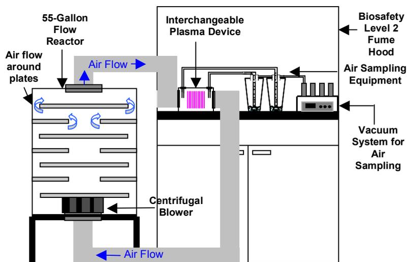
Figure 4. Pathogen Detection and Remediation Facility (PDRF)
