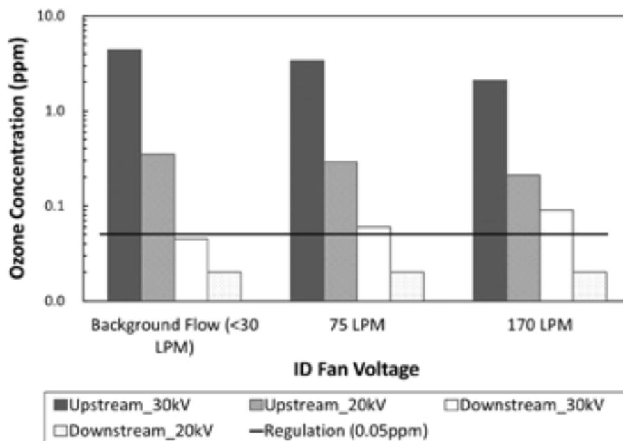
**Figure 9.** Measured ozone concentration upstream and downstream of the single layer ozone filter with either 20kV or 30kV power supply at varied air flow rates. The dashed line represents the ozone standard for indoor air cleaners set by the state of California [31].
