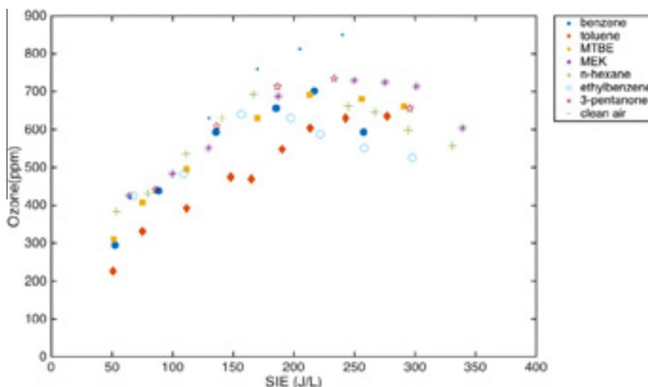
Fig. 4. SIE impact on effluent ozone concentration at a flow rate of  $6.6 \text{ L min}^{-1}$ . Typical standard deviations for the ozone measurements were 40–60 ppm<sub>v</sub>.
