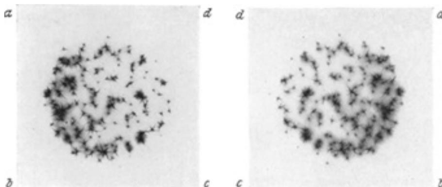
Fig. 2. Photographic footprints of current filaments [55].
