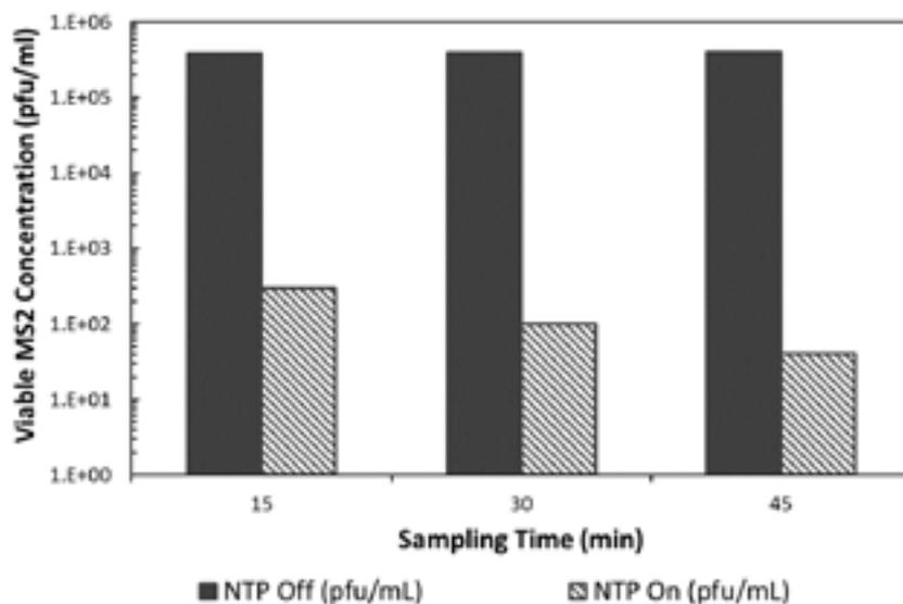
**Figure 5.** Change of infectious MS2 concentration in the downstream impinger with either ozone-free air (reactor off) or ozone-loaded air (reactor activated by 20kV) bubbling through the impinger liquid.
