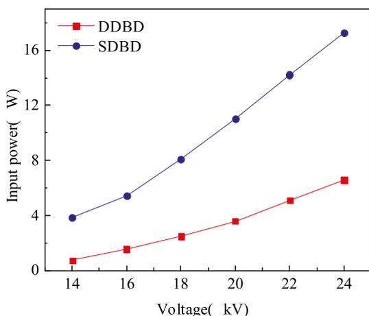
Fig. 8. The input power of DDBD and SDBD.
