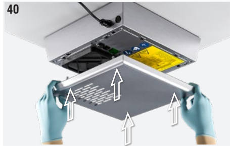
Fig. 40: Replace the external cover by fixing it to the pins.
