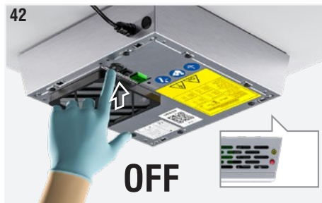
Fig. 42: Turn the device off by turning the O/I switch to the 0 position.
