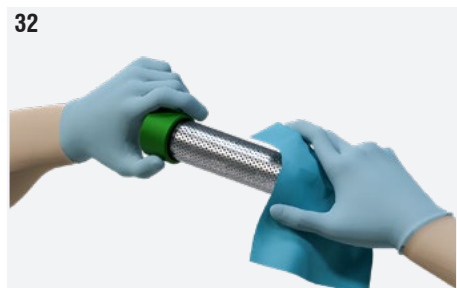
Fig. 32: Clean the glass using a damp cloth.
