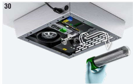
Fig. 30: Gently unscrew the ionizing tube by grasping it at the base (green part).
