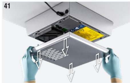
Fig. 41: Remove the external cover by grasping it sideways and pulling to release it from the device.
