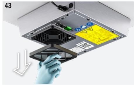
Fig. 43: Remove the filter cover by pressing the sides and pulling towards you.
