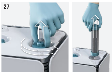
Fig. 27: Gently unscrew the ionising tubes by acting on the safety cup that can be reached by hand through the special slots.
