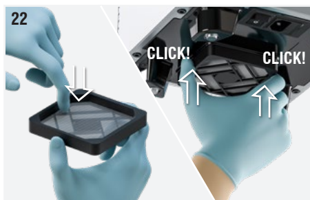
Fig. 22: Put the mesh filter back into the filter cover. Reassemble the filter cover with the snap fastening. Press it on the grid incorporated in the closing plate until you feel the snap of the coupling between the parts.
