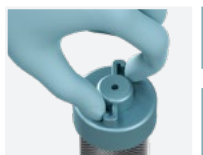
Fig. 13: Clean the tube with a slightly damp cloth (that does not shed fibres), slightly rotating the metal mesh around the glass.
