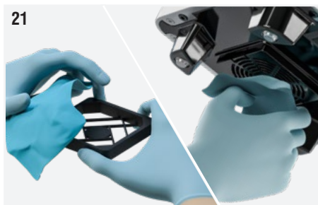
Fig. 21: Use a damp microfibre cloth to wipe the plastic filter cover and the grid incorporated in the closing plate.
