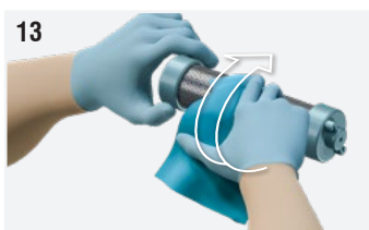
Fig. 13: Clean the tube with a slightly damp cloth (that does not shed fibres), slightly rotating the metal mesh around the glass.
