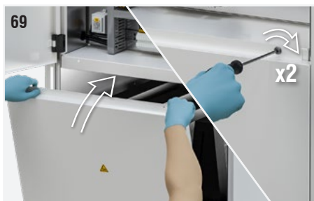
Fig. 69: Put the cover panel back in place. Screw the screws back on.
