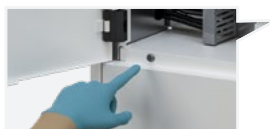
Fig. 66: Unscrew the 2 screws which keep the rear bottom panel for maintenance access. Lift and then pull you towards to remove the panel.
