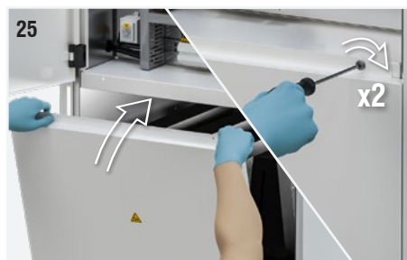
Fig. 25: Put the cover panel back in place. Screw the screws back on.
