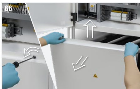
Fig. 66: Unscrew the 2 screws which keep the rear bottom panel for maintenance access. Lift and then pull you towards to remove the panel.
