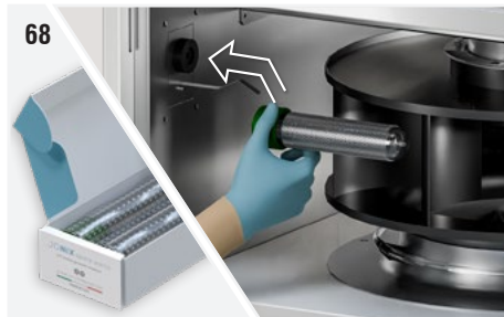
Fig. 68: Gently screw in the new ionising pipe , holding on to the base (green part). If the operation is difficult to perform, pull slightly the earthing spring so that it is not in contact with the surface of the tube.
