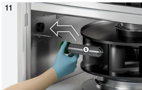
Fig. 11: Gently tighten the ionising pipe by gripping it at the base (green part), positioning it in its seat above the fan. If the operation is difficult to perform, pull slightly the earthing spring so that it is not in contact with the surface of the tube.
