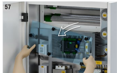
Fig. 57: Unscrew the knobs and remove the internal plexiglass panel to access the ionizing tubes.
