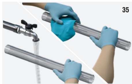
Fig. 35: Wash the mesh under running hot water and dry it thoroughly with a non-fraying cloth.
