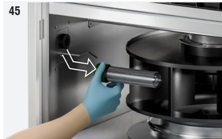
Fig. 45: Gently unscrew the ionising pipe, gripping it at the base (green part). If the operation is difficult to perform, pull slightly the earthing spring so that it is not in contact with the surface of the tube.
