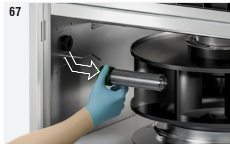
Fig. 67: Gently unscrew the ionising pipe, gripping it at the base (green part). If the operation is difficult to perform, pull slightly the earthing spring so that it is not in contact with the surface of the tube.
