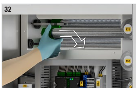
Fig. 32: Gently unscrew the ionising pipe, gripping it at the base (green part). If the operation is difficult to perform, pull slightly the earthing spring so that it is not in contact with the surface of the tube.
