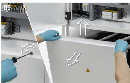
Fig. 9: Unscrew the 2 screws which keep the rear bottom panel for maintenance access. Lift and then pull you towards to remove the panel.
