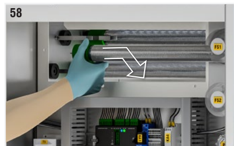
Fig. 58: Gently unscrew the ionising pipe, gripping it at the base (green part). If the operation is difficult to perform, pull slightly the earthing spring so that it is not in contact with the surface of the tube.
