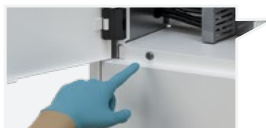
Fig. 9: Unscrew the 2 screws which keep the rear bottom panel for maintenance access. Lift and then pull you towards to remove the panel.
