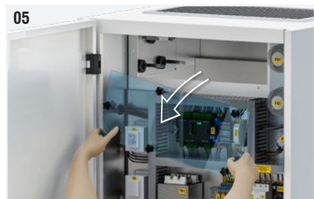
Fig. 5: Unscrew the knobs and remove the internal plexiglass panel to access the ionizing tubes.
