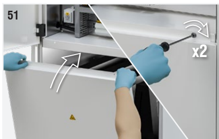
Fig. 51: Put the cover panel back in place. Screw the screws back on.
